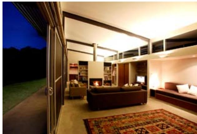
Interior of residence with good cross ventilation, thermal mass in an exposed concrete slab floor, and low VOC (volatile organic compounds) finishes
